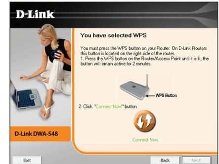
Press the WPS button on your access point or wireless router within 2 minutes to establish connectivity.
